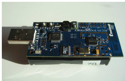
Figure 3.18: TmoteSky sensor node.
