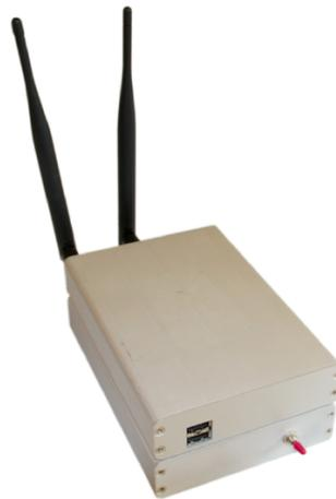
**Figure 6.9:** Prototype of a battery-powered OViS WMN node.
