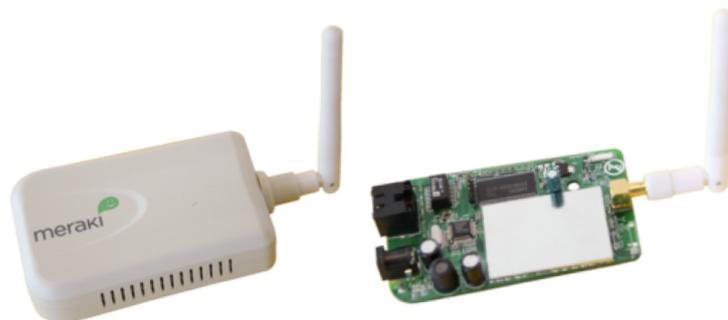
**Figure 2.5:** Meraki Mini with an indoor case.
