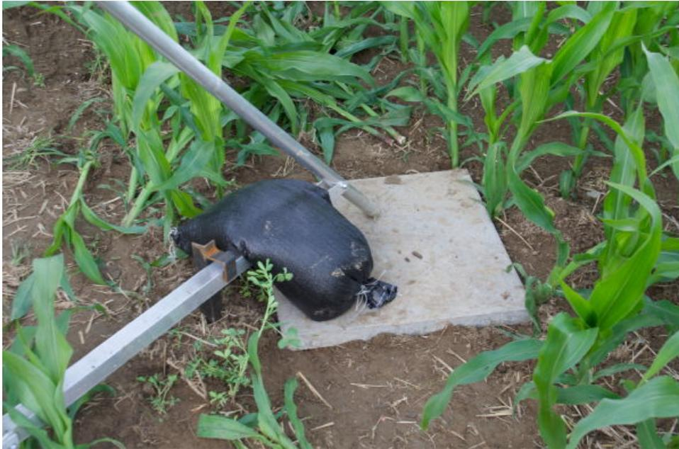
**Figure 5.11:** Concrete paving slab to prevent sinking in of the tripod, sand bag and iron stake to stabilise mast.
