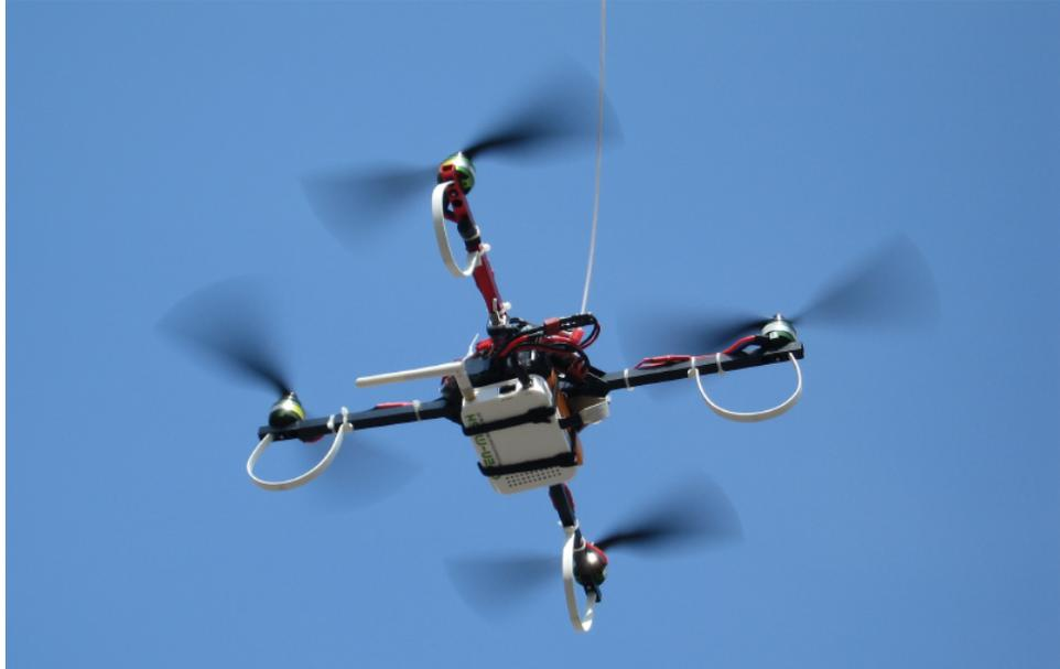
**Figure 7.7:** Flying quadcopter UAV carrying a WMN node.
