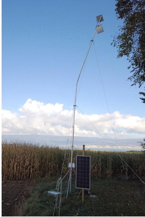
**Figure 5.13:** Broken mast due to strong winds and loose guying (*node02*).
