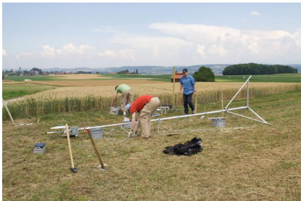
**Figure 5.10:** Complete assembly of telescopic mast in horizontal position before final setup.
