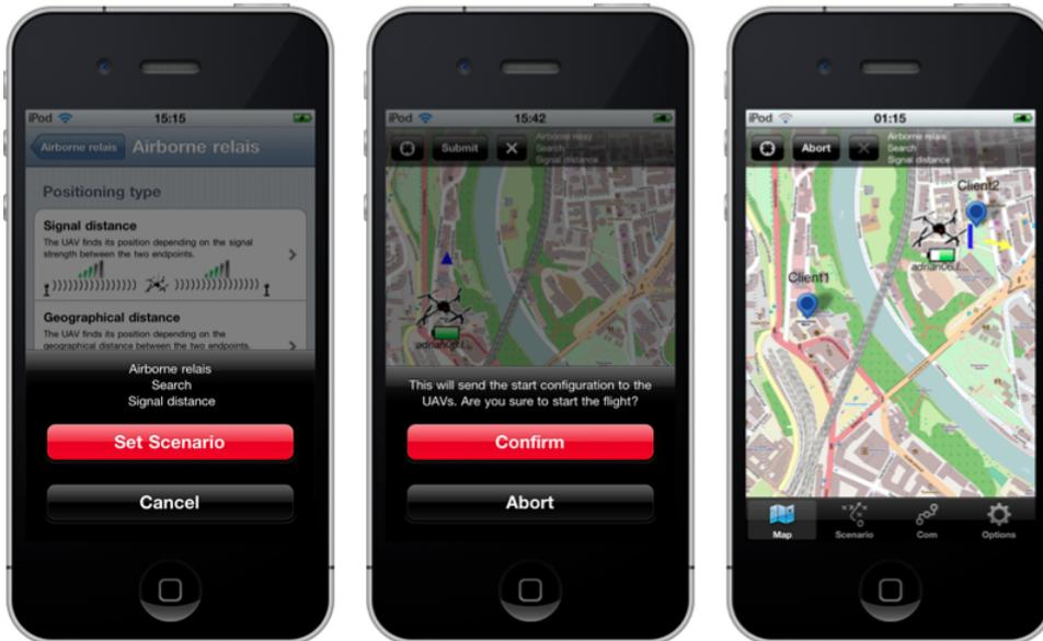
**Figure 7.12:** Remote Control Application (iPhone): setting the scenario, confirmation, and monitoring of flying UAVNet.
