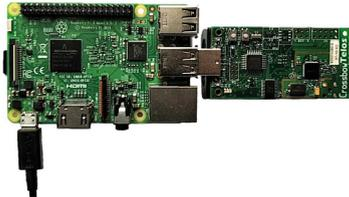
**Fig. 2.** Border router with Raspberry Pi and TelosB
