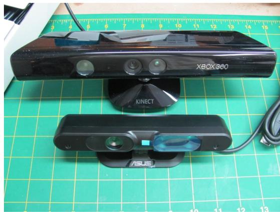
**Figure 3.10:** Size comparison between Kinect and Xtion[50]
