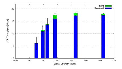
Figure 6.3: UDP throughput between two mesh nodes depending on signal strength.
