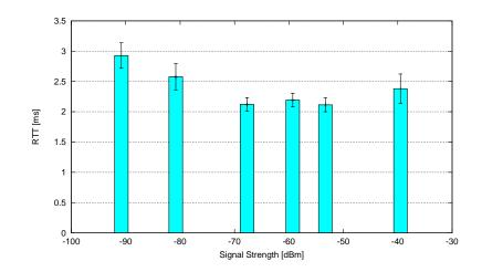
Figure 6.4: RTT between two mesh nodes depending on signal strength.
