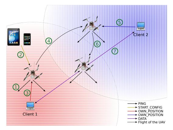
Figure 3.9: Procedure of the Location Positioning mode.
