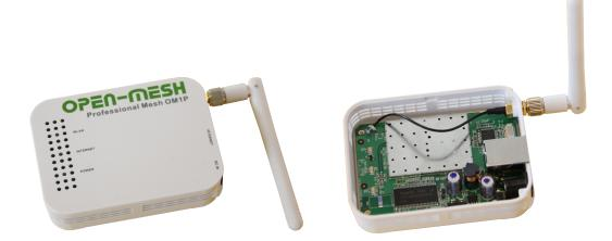
Figure 2.4: Professional Mesh Node OM1P from Open-Mesh [6].
