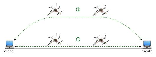
Figure 6.11: End-to-end throughput setup using a Multi-hop Airborne Relay scenario.
