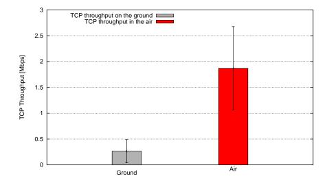
Figure 6.12: TCP throughput between two notebooks in a multi-hop airborne relay setup.
