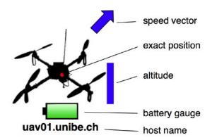
Figure 2.9: Current state of a UAV in the Remote Control App [6].
