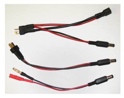
Figure 4.2: Different cables to provision electric power to the UAV and the mesh node.
