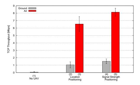
Figure 6.10: TCP throughput between two notebooks in an airborne relay setup.
