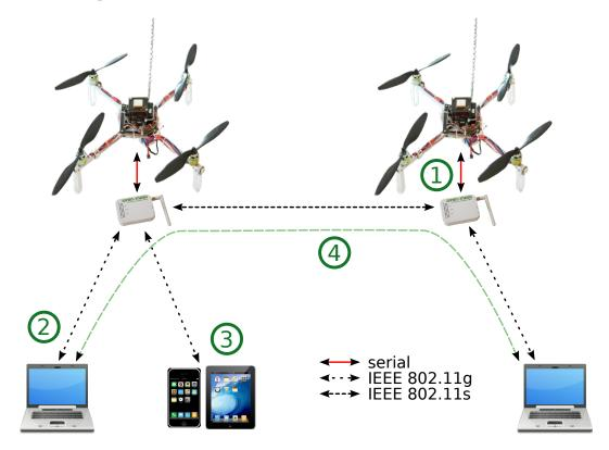
Figure 3.1: Typical setup of *UAVNet* with two UAVs with attached wireless mesh nodes and multiple clients.
