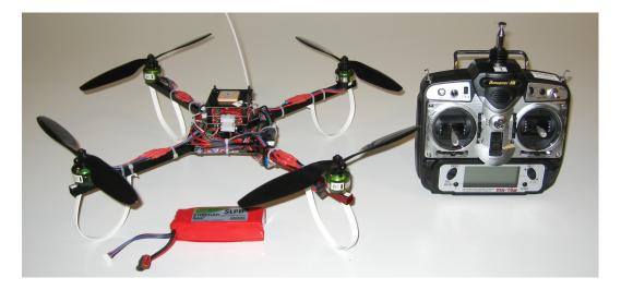
Figure 2.2: Assembled Mikrokopter kit.
