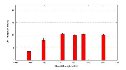
Figure 6.2: TCP throughput between two mesh nodes depending on signal strength.
