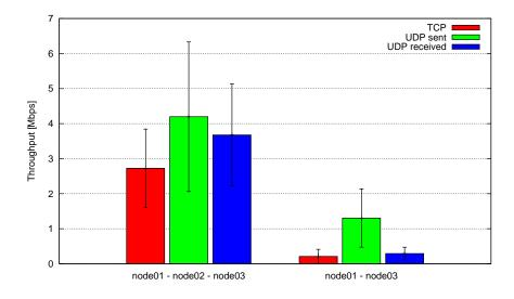
Figure 6.8: TCP and UDP throughput over multiple mesh nodes.
