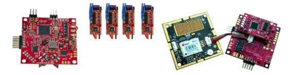
**Figure 2.3:** Flight electronics of a Mikrokopter (from left to right): the main controller board FlightCtrl, brushless controllers, GPS board and the navigation controller board NaviCtrl with an attached three dimensional compass [6].
