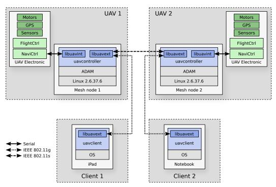
Figure 3.2: Architecture and communication interfaces of UAVNet.
