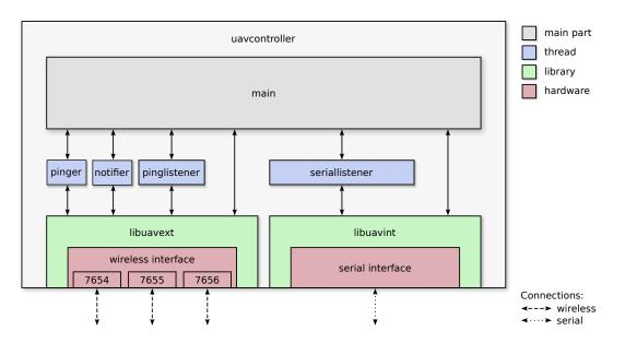
Figure 5.2: Schema of the architecture of the *uavcontroller*.
