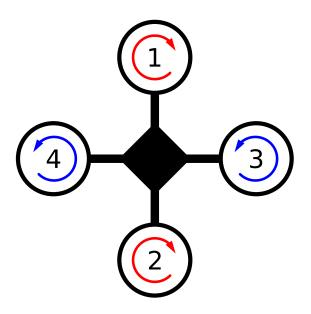
Figure 2.1: A quadrocopter's principle of flight.
