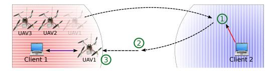
Figure 3.5: Multi-hop Airborne Relay scenario: setup UAV 1.
