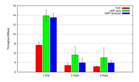
Figure 6.6: TCP and UDP throughput over multiple mesh nodes.
