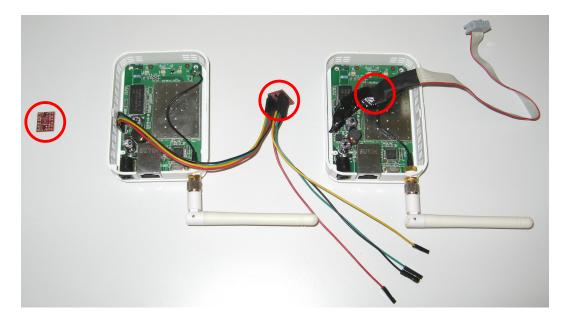
Figure 4.3: Logic Level Converter during the development phase and in the final prototype implementation.
