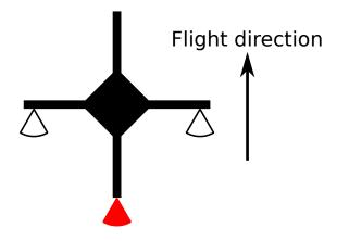
Figure 4.1: Used lighting scheme of a UAV.
