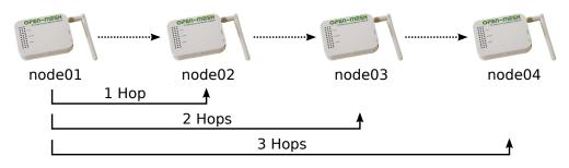
Figure 6.5: Evaluation Setup of Multi-Hop Performance Measurements.
