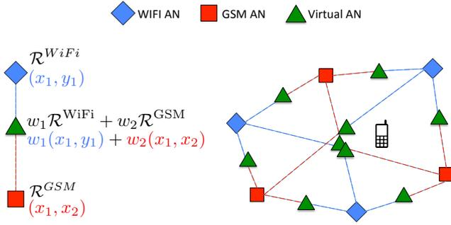
Figure 4: Construction and placement of VANs
