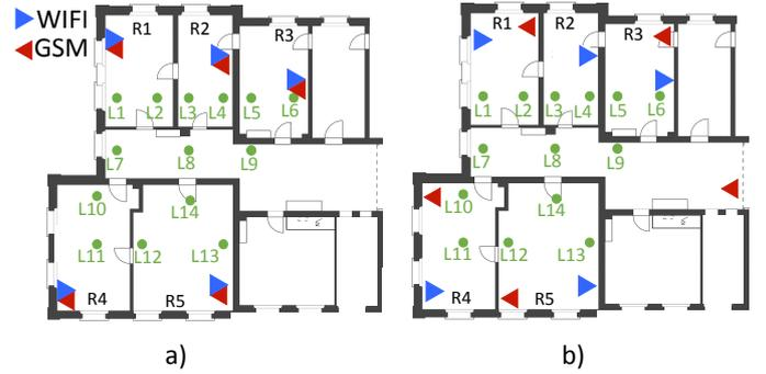
Figure 5: a) colocated antennas setup. b) distributed antennas setup
