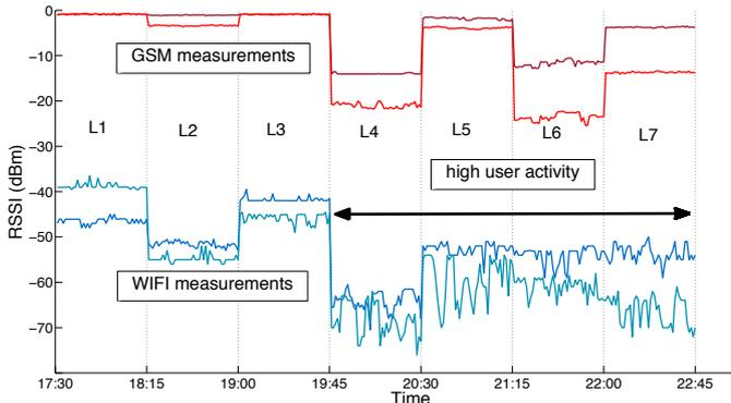
**Figure 7: Comparing Signal Interference for collocated Antennas**
