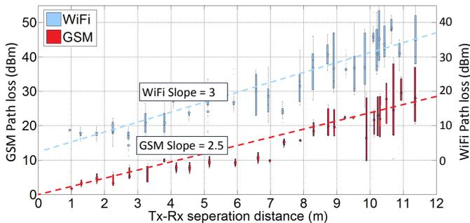
Figure 8: Comparing WiFi and GSM path loss
