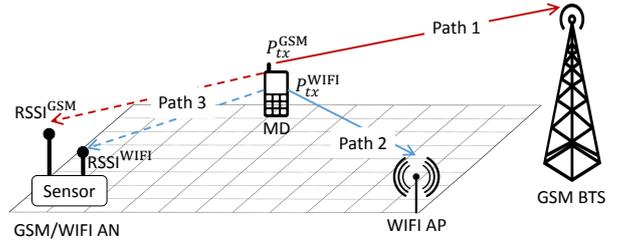
Figure 1: Signal overhearing setup
