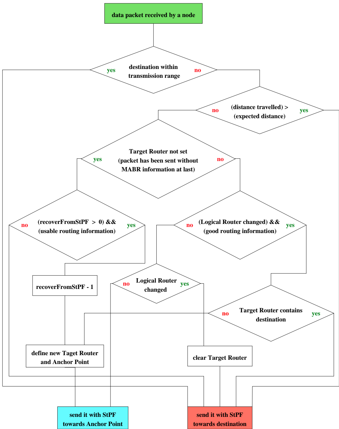
Figure 4.10: Flowchart for redirecting of a data packet
