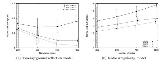
Figure 5.19: Overhead with isotropic and irregular transmission ranges
