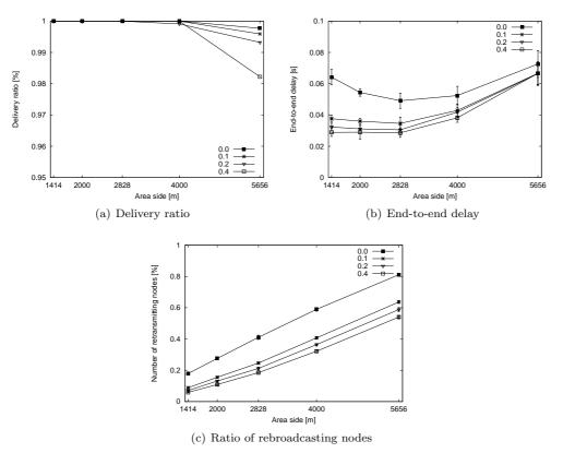
Figure 6.11: Impact of rebroadcasting threshold RT
