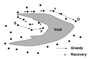
Figure 3.8: Suboptimal path taken by position-based routing protocol
