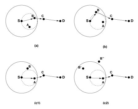
Figure 5.5: Routing with BLR in unicast mode
