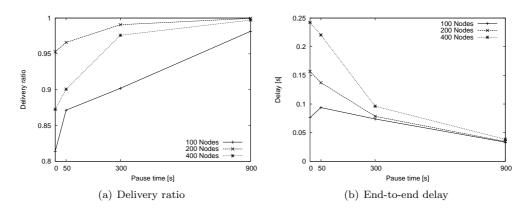
Figure 4.3: Performance of GFG/GPSR with varying mobility and node density
