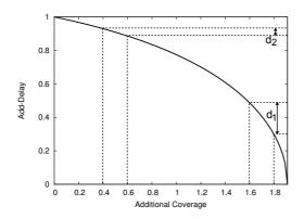
Figure 6.3: Delay introduced by the DFD function
