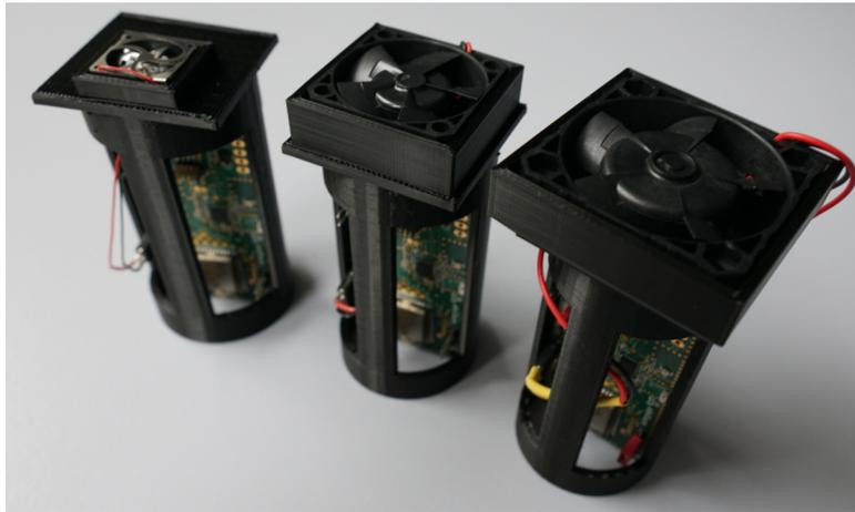
Figure 6.4: 3D printed frames used to mount the PCB and fan inside the housing
