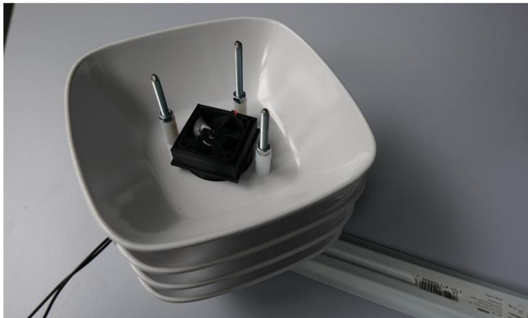
Figure 6.5: Upside down view of the prototype with the bottom bowl removed clearing the view onto the 3D printed frame with the medium fan installed
