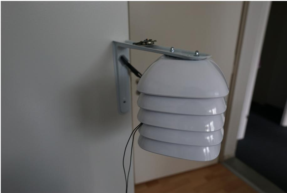
Figure 8.1: Test setup with the sensor prototype mounted indoors
