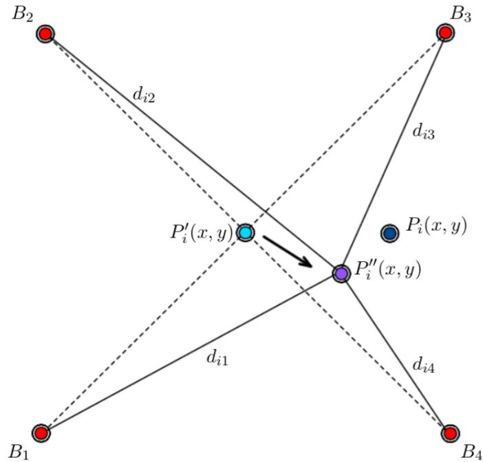
**Figure 3.5:** Exemplification of centroid and weighted centroid localization.
