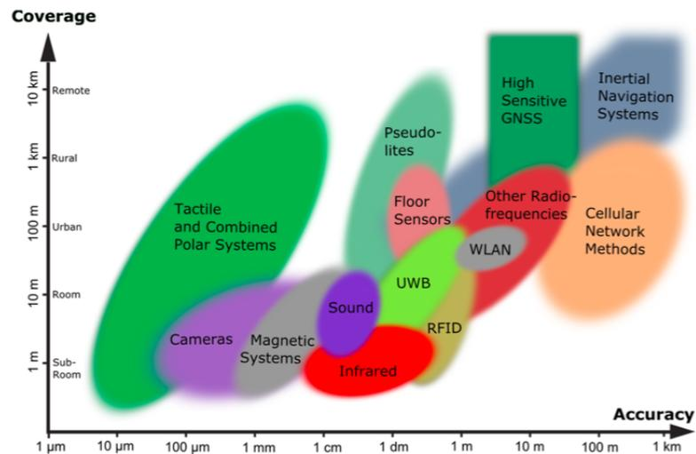
**Figure 2.2:** Overview of indoor positioning technologies in dependence on accuracy and coverage [2].
