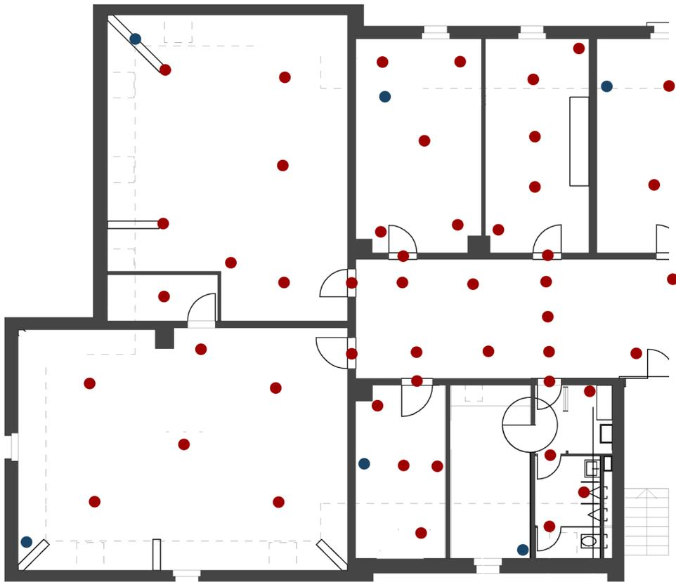
FIGURE 5.2: Floorplan of the testing environment. Blue dots denote WiFi access points, red dots locations at which samples were taken.
