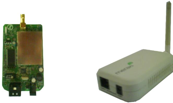
**Figure 1.2:** Meraki Mini node hardware with indoor case
