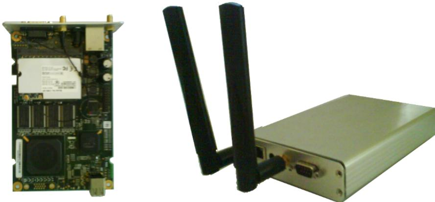
**Figure 1.3:** PC Engines Alix node hardware with indoor case
