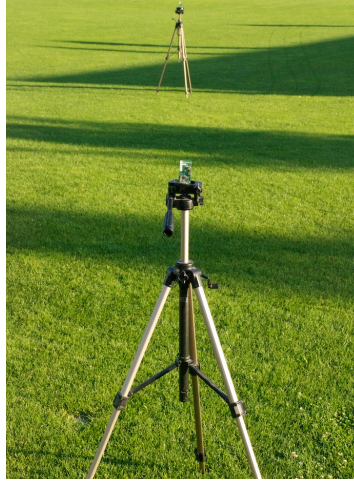
Figure 3.8: TelosB node on tripod in outdoor testbed.
