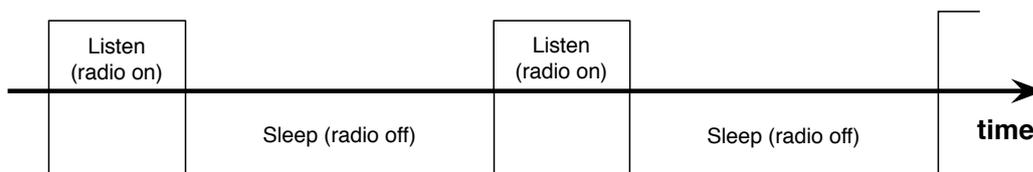
**Figure 2.2:** Listen/sleep cycles in S-MAC. During the sleep cycle the radio is completely to save energy.
