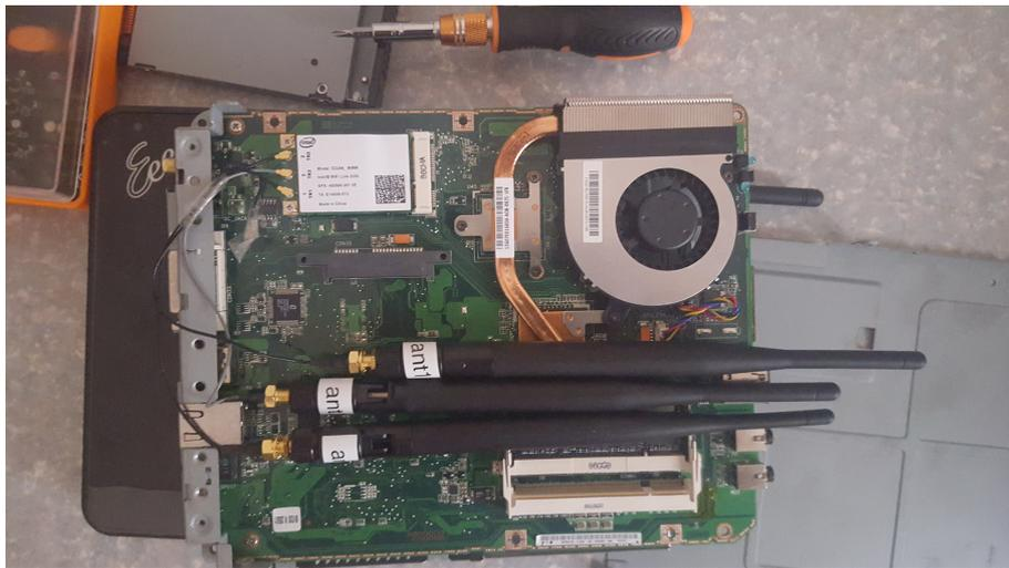
**Figure 5.4:** Disassembled ePC with antennas (part two)
